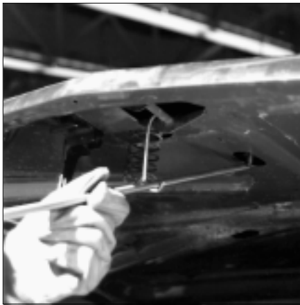
Figure 2—Paintless dent repair requires prying from the panel backside by inserting pry tools in access holes.
