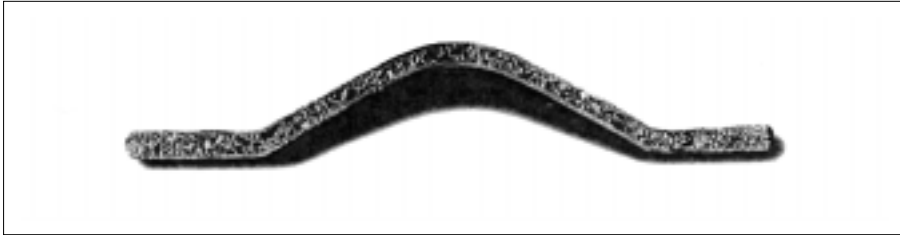
Figure 1—A new method of making foam sandwich panels enables the panel to be formed into complex shapes. (Courtesy of Karmann USA, Inc.)
