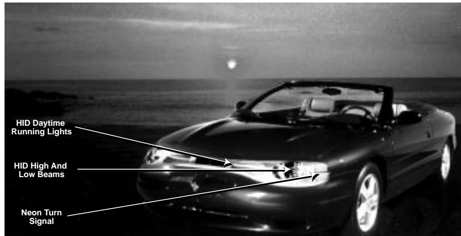
High- and low-beam HID headlamps and neon auxiliary lamps are two innovative lighting ideas shown on this vehicle. (Courtesy of Osram Sylvania, Inc.)
