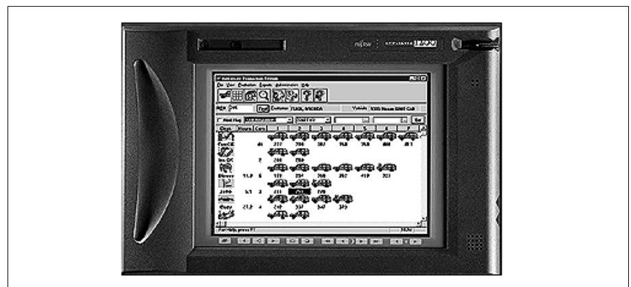
Figure 4—This screen is shown on a laptop computer that can be taken to the back lot to check on the progress of repairs. Written comments can be made with a light pen. (Courtesy of Mitchell, Inc.)
