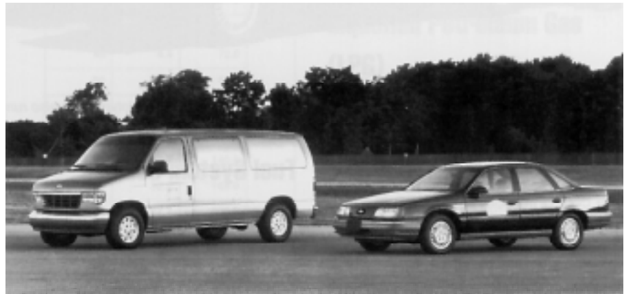
Ford has converted a fleet of Econoline vans and Tauruses to flexible-fuel vehicles that use methanol, gasoline, or any combination, from the same tank. (Photo courtesy of Ford Motor Company)
