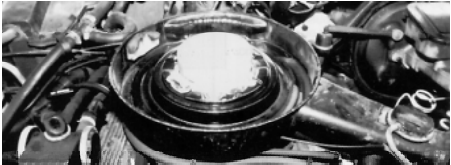
Figure 9—The CNG mixer on this V8 Chevrolet Caprice fits inside the air cleaner housing.
