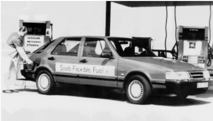
Figure 1—Most engines designed to run on methanol, such as this Saab prototype, can also run on gasoline or any combination of the two. (Photo courtesy of Saab Cars USA, Inc.)
