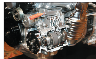
Figure 1 – In this cutaway of the "hybrid" dual-scroll air conditioning compressor, the size difference is evident between the larger belt-driven front compressor and the smaller electric motor driven rear compressor. (Courtesy of American Honda)
