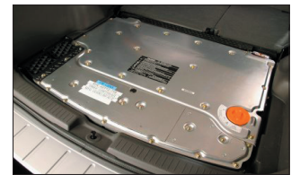
Figure 3—The high voltage battery is located in the rear cargo area.
