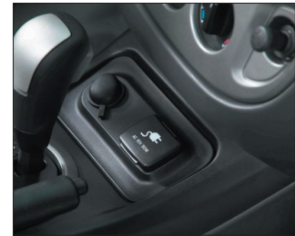
Figure 4—The optional 110-volt outlet on the center console.
