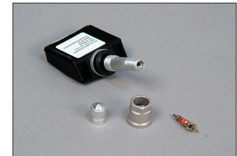
Figure 2—TPMS sensors may be attached to a special tire valve.
