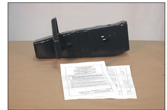
Figure 1—This part can be ordered to section the front frame on the 2004 Ford F-150.
