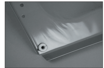
Figure 1—Stretch marks on this aluminum sheet metal part indicate a stamping operation.
