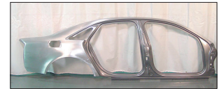
Figure 4—This one-piece stamping is the uniside on the A8.
