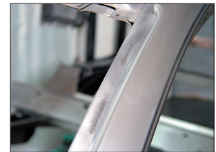
Figure 5—The thin, straight weld joints on this A-pillar are robotic laser welds.
