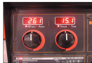
Figure 3—The easy to read digital display on the Lincoln Power MIG 300 allows precise adjustment for welder setup.
