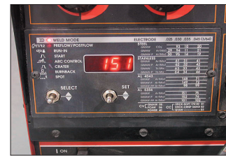
Figure 2—Multiple parameters and programs on the Lincoln Power MIG 300 allow the technician to adjust the welder to the specific job.
