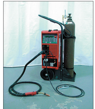
Figure 1—The Fronius TPS2700 digital GMA (MIG) welder is a programmable computer-controlled welder for use on aluminum.
