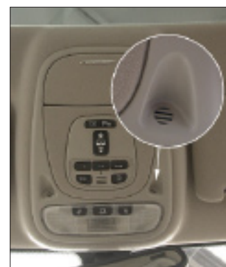
Figure 1—The seat occupant sensor, as shown on this 2003 Jaguar XJ, monitors the position and height of the passenger to help the control module determine if the airbag should deploy.
