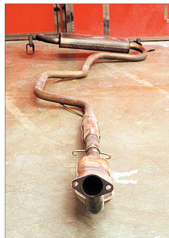
Figure 1— This is an example of a welded, one-piece exhaust system.
